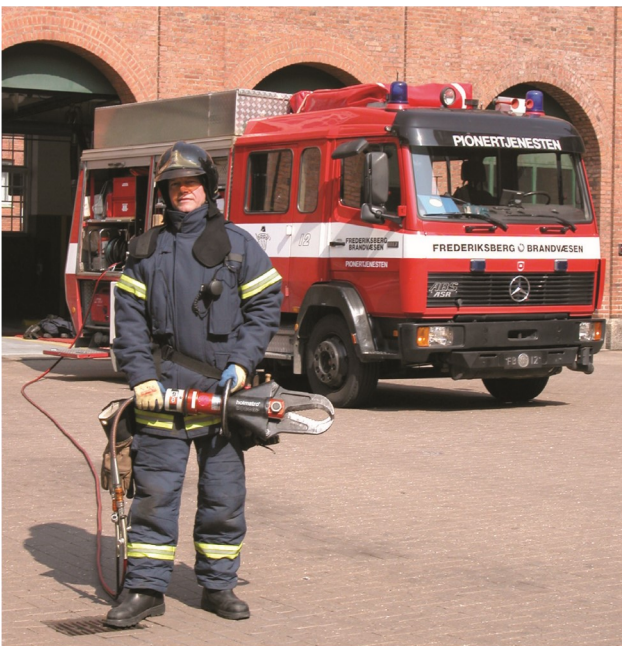
Tools can be operated 40 meters away from Rescue truck with help of hoses.
