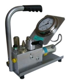
Manufacturing and performing safety maintenance on big cranes demand the tensioning of several big bolts. Hydraulic bolt tensioners are often used to ensure high-quality assembly and good homogeneity. The tensioners can be powered fast and easy, by tapping into the crane system hydraulics, boosting the 160 bar, with a miniBOOSTER, to achieve up to 1,500 bar, which is necessary for tensioning the big bolts. Compared to an air-driven Power Pack, this solution is up to 5 times faster.
